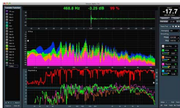
Smaartv7 (beta) TopPane:Live IR; MiddlePane:4x Live RTA; Bottom Pane:4x Live Transfer Function
